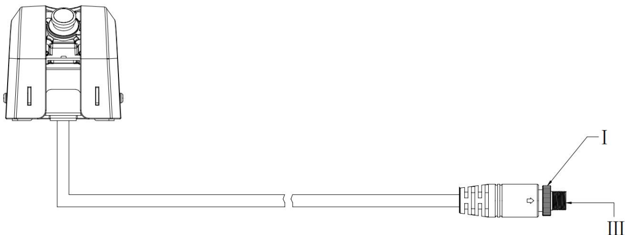
M12 waterproof connector---default 0.5 meters (tail length)
